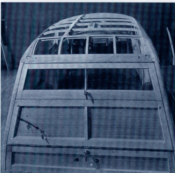
An October 1940 Pontiac Torpedo advertisement (opposite) included a station wagon in the lineup. The Hercules bodies (above and left) used Honduras mahogany inset panels in a white ash frame work.
