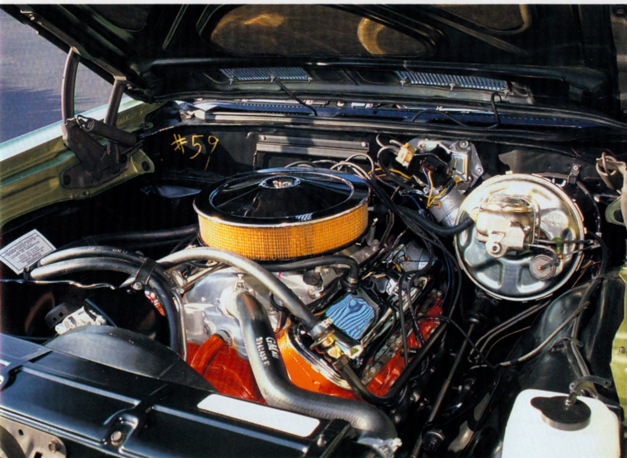
The 1969 Chevelle COPO 9562 (below) was powered by a cast-iron L-72 427cid high-performance engine (above).
