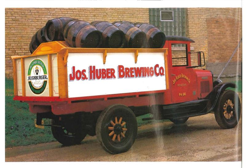
The Six-Speed Special (above) was rated at one-ton capacity. Although its 173-cid Waukesha engine turned out only 30 horsepower, the use of pneumatic tires and the two-speed rear axle combined to push the truck to a top speed of over 45 miles per hour-quite good in the days when most roads were still narrow, hilly, and curvy. The closed cab (opposite page), primitive by today's standards, featured roll-down side windows, a fold-out windshield, and a big steering
