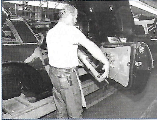
Twenty-two year employee Don Hazelwood installs the passenger door panel. At the same station, Bob Love, a 23-year veteran, installs the interior trim panels. Once it leaves their station, it will receive interior carpeting, rear speaker covers and console side covers.
