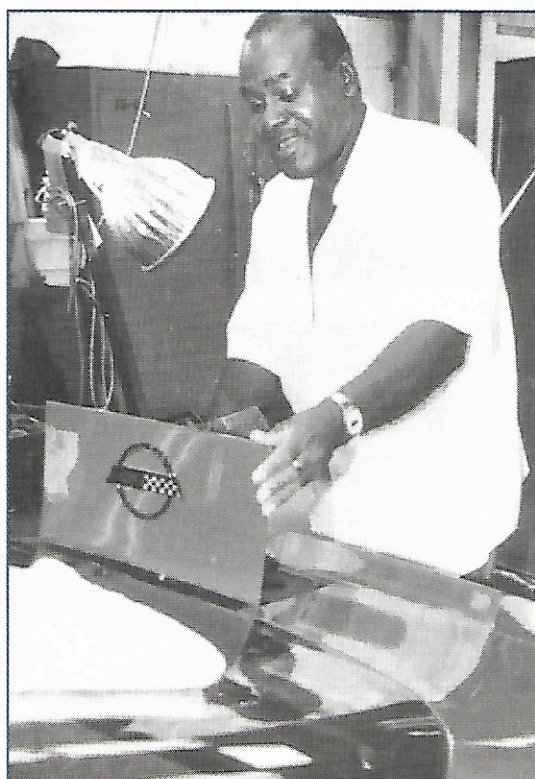
After the water leakage test, the ZR-1 goes to the "finesse line." Convertible tops receive a protective plastic cover. The finesse line is the last opportunity to inspect the paint finish for flaws under extremely bright lights. If any defects turn up, the paint is gently cut and then repolished to see if the defect is repaired. If the fault can't be repaired here, the car is pulled off the line and taken to an adjacent area for paint repair. If the car passes, it stays on the finesse line and moves through a wash booth. Once washed, paper mats are placed on the floor and the paint is glazed. Floyd Channel, a 24-year GM employee and owner of an 1981 Corvette, places the fuel door emblem on the ZR-1 while up front Danny Bruce installs the hood emblem and the underhood "Built In Bowling Green" plaque. From there, the ZR-1 is sprayed with a protective coating in a small, garage-sized spray building right next to the plant exit.
