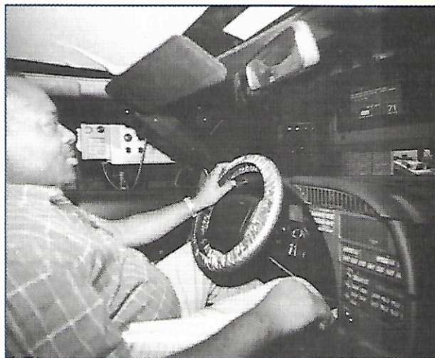
From the alignment pit, the car is driven to the DVT (Dynamic Vehicle Test) booth, a computerized check of all vehicle functions. After plugging the test computer into the ALDL plug under the instrument panel, George Ford types in the Corvette's VIN and the computer takes the ZR-1 through its paces. The DVT will test the air conditioning system, transmission up and down shifts, ECM, cruise control and other functions. George follows prompts from the computer on a TV monitor, telling him, for example, when to apply throttle and at what rpm.
