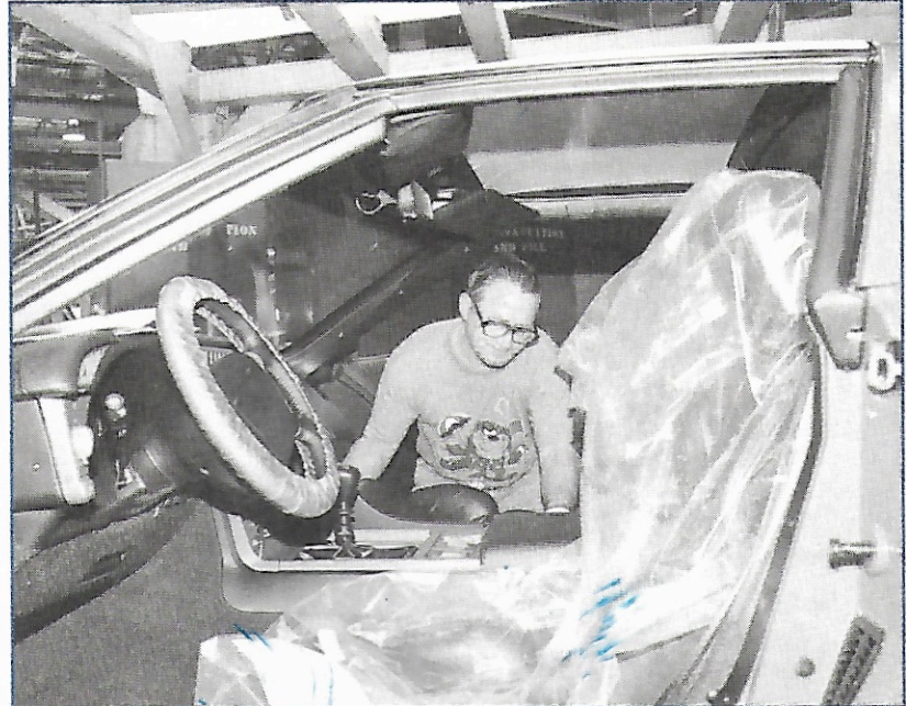
Since some interior components had to be installed in inaccessible areas first, the knee bolsters and seats can now be bolted in. E.C. McKenzie slips the passenger seat into the ZR-1 after installing the seat track.
