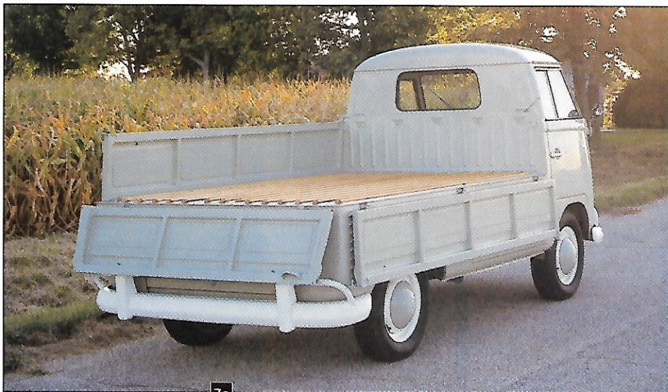
7. The vehicle that influenced the Econoline pickup was the Volkswagen Type 2. Because of its rear engine design (7a), the box sits considerably higher than the Ford's. Volkswagen designed fold-down sides and incorporated individual under-the-floor cargo compartments to utilize the remaining space to its full extent. Chevrolet's rear-engined Corvair Rampside retained the lower cargo deck, and raised only the area over the engine compartment. This nicely restored 1961 VW pickup is owned by Brian Holcomb, Watertown, Wis.
